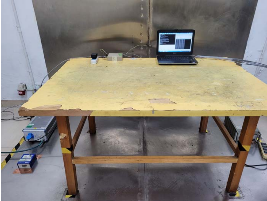
Conducted Emission Front View
