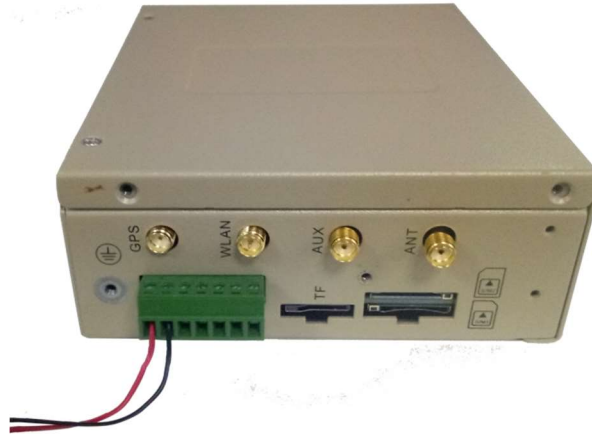
Figure 3-7 Installing the Power Supply
