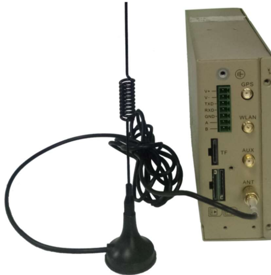
Figure 3-6 Installing an Antenna
