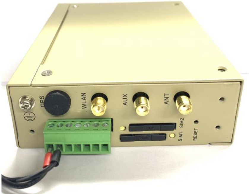
Figure 3-5 Installing the Power Supply
