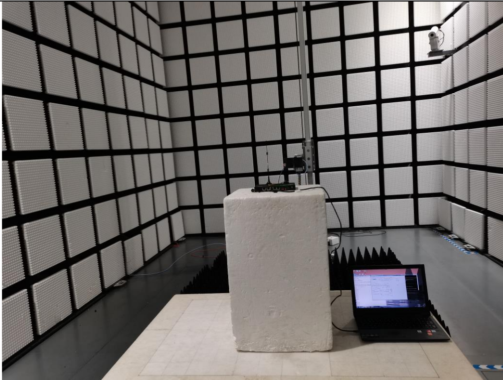
Radiated emission setup photo(Above 1GHz)
