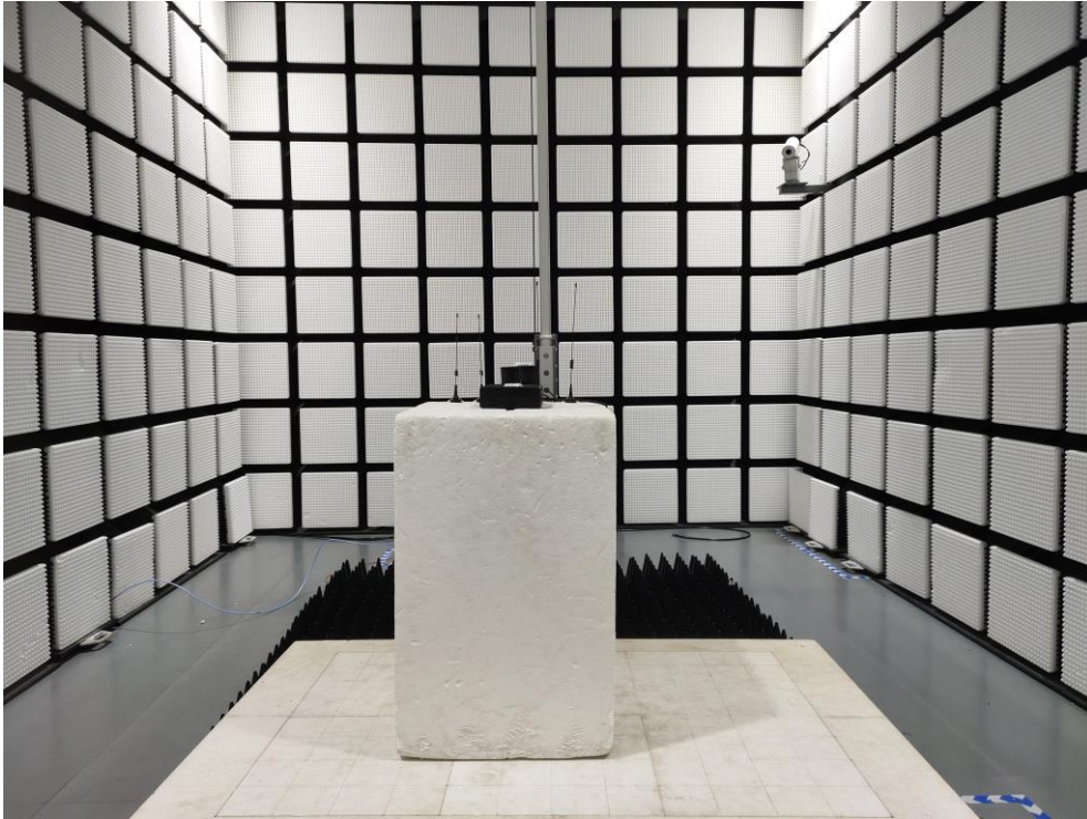
Fig. 3 Radiated emission setup photo(Above 1GHz)
