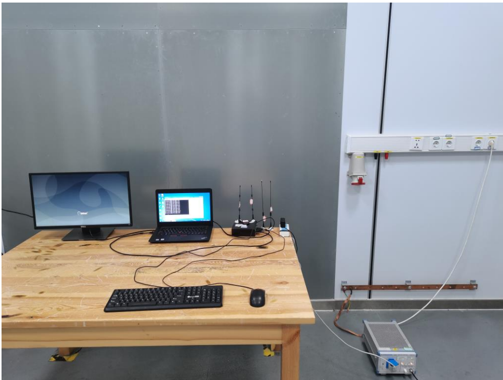
Fig. 4 Power line conducted emission setup photo
