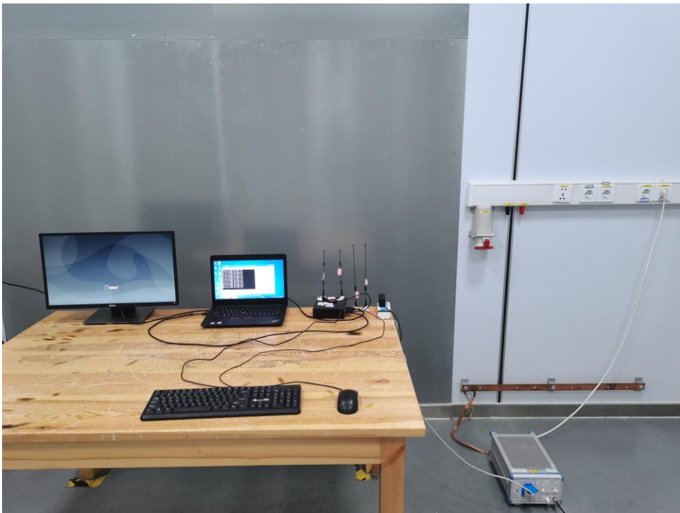
Fig. 4 Power line conducted emission setup photo
