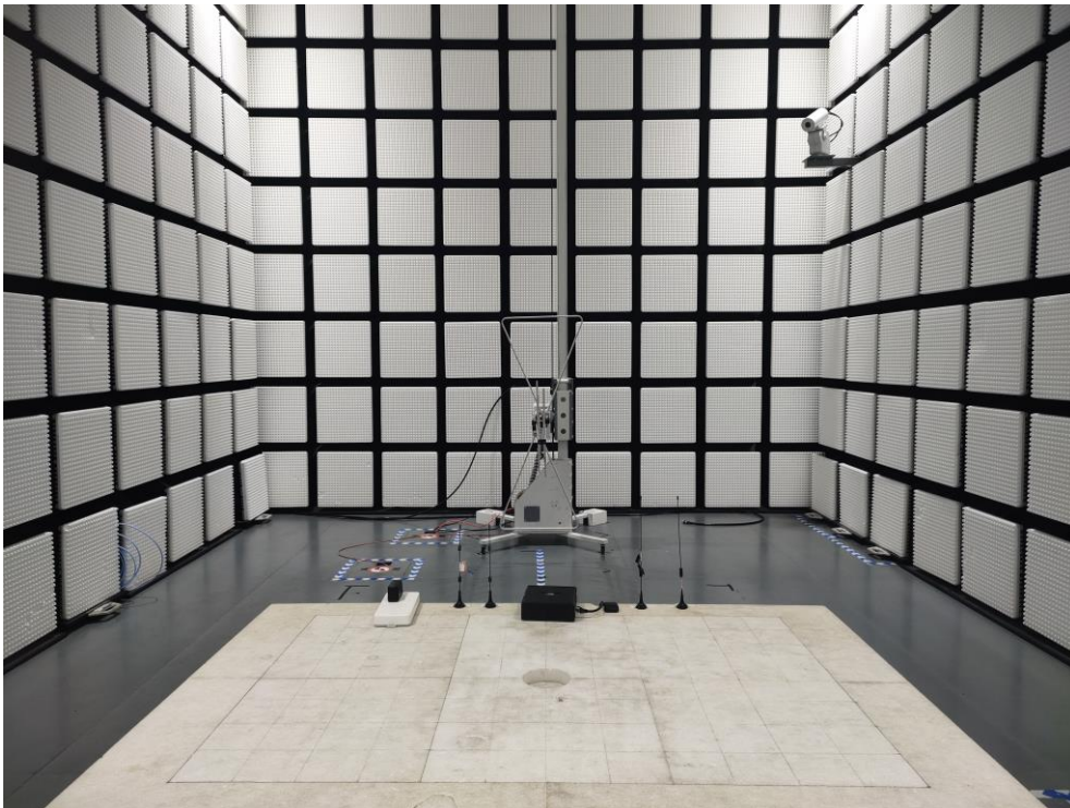
Fig. 2 Radiated emission setup photo(30MHz-1GHz)
