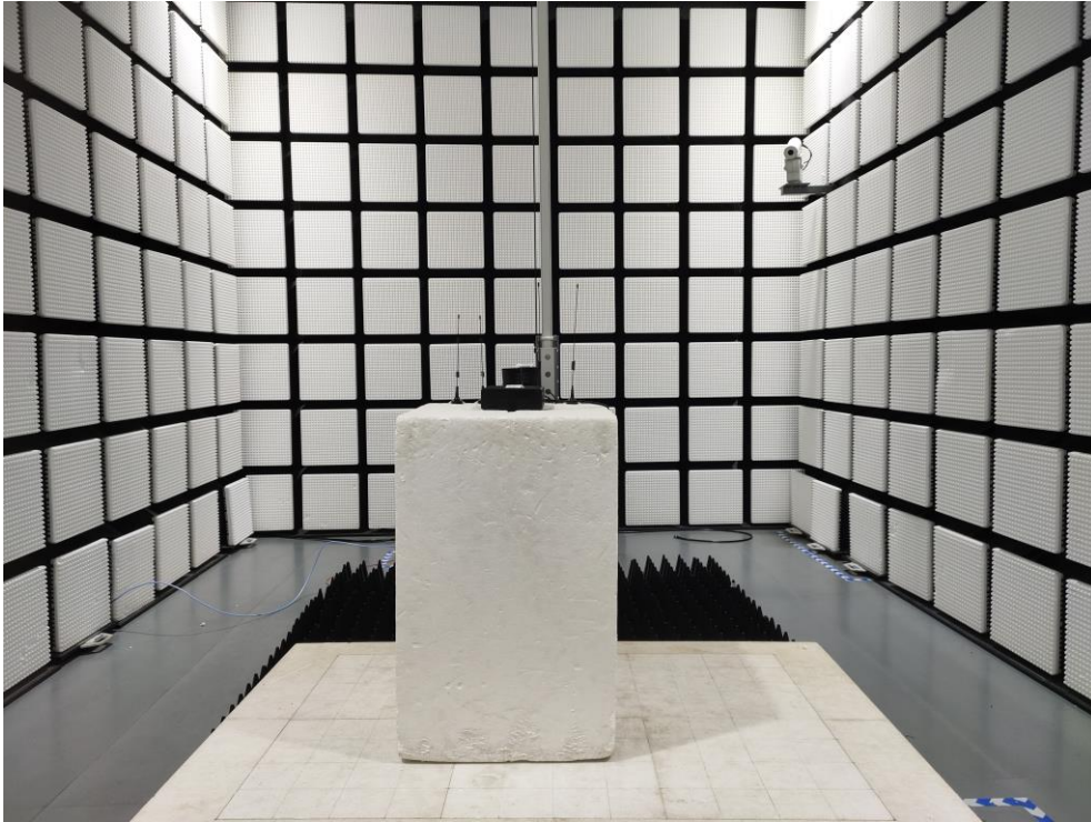
Fig. 3 Radiated emission setup photo(Above 1GHz)
