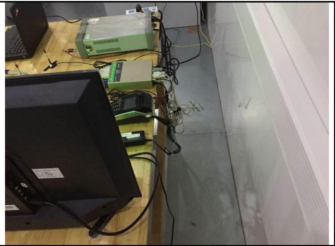
Conducted Emissions Test Setup – Rear View
