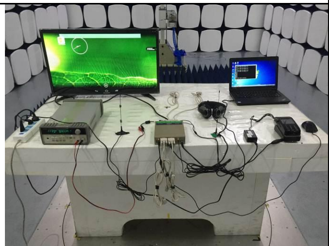
Radiated Spurious Emissions Test Setup Above 1GHz
