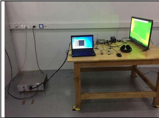
Conducted Emissions Test Setup – Front View
