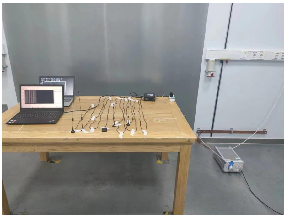
Fig. 4 Power line conducted emission setup photo
