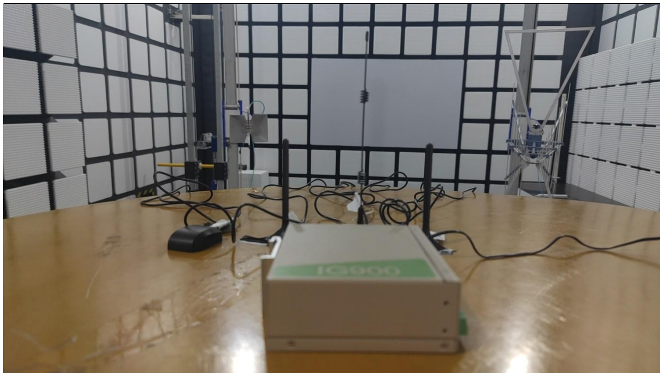
RF Radiated Test setup (RSE)
