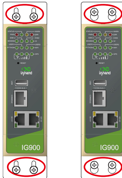
Figure 3-4 Wall mounted installation diagram
