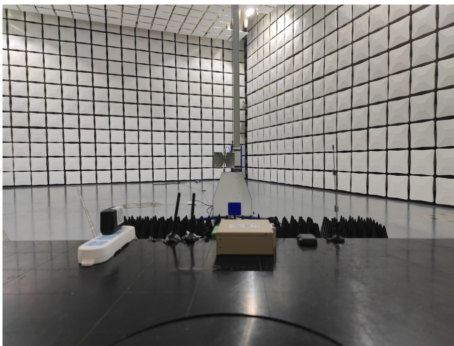
Radiated Emissions Test Setup (with charger) (above 1GHz)
