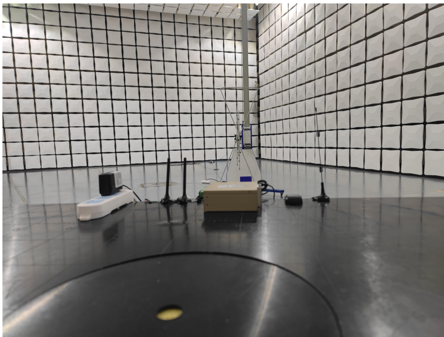
Radiated Emissions Test Setup (with charger) (30-1000MHz)
