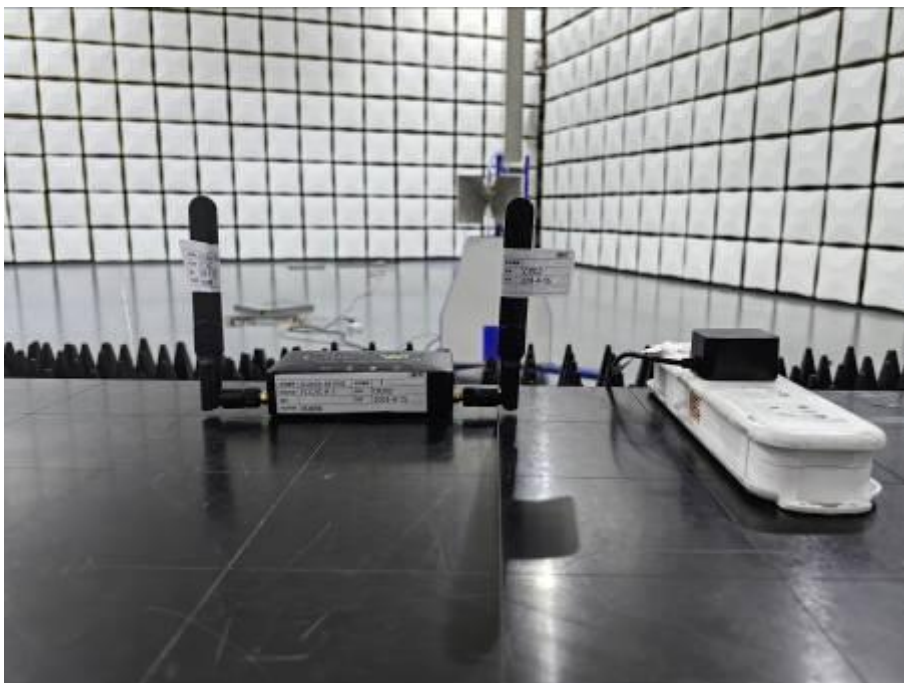
Radiated Emissions Test Setup (above 1GHz)
