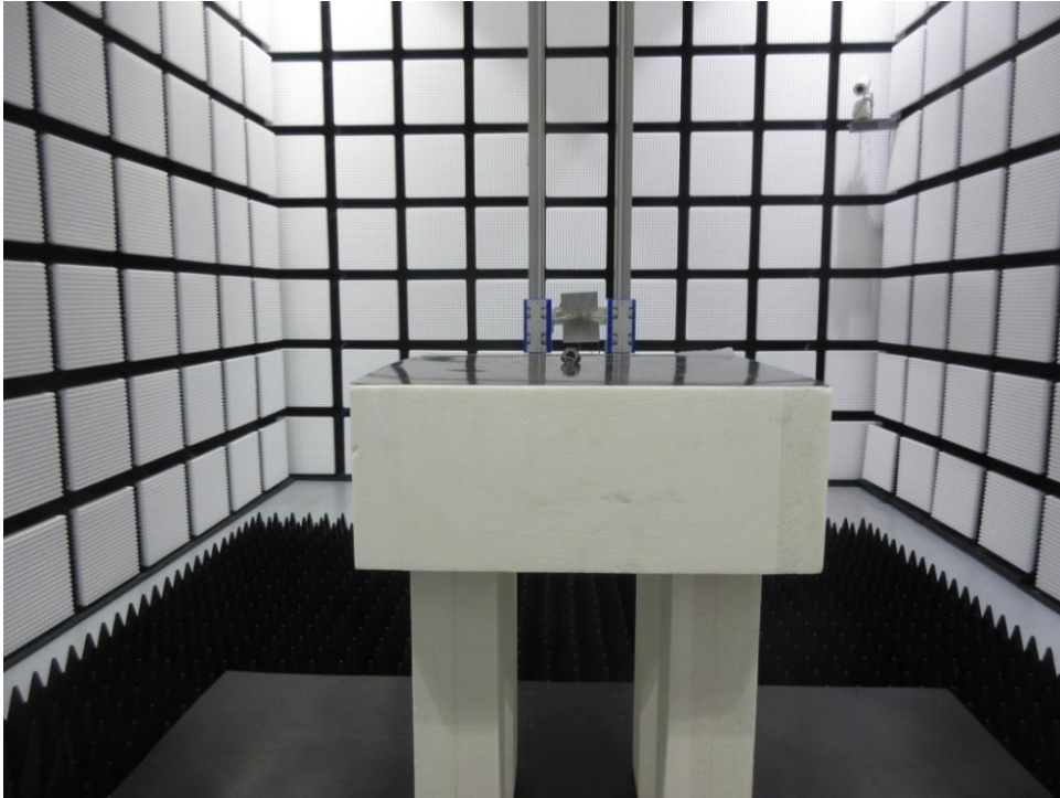
Radiated Emission test Above 1GHz
