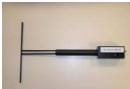
Figure 1 – Satimo COMOSAR Validation Dipole
