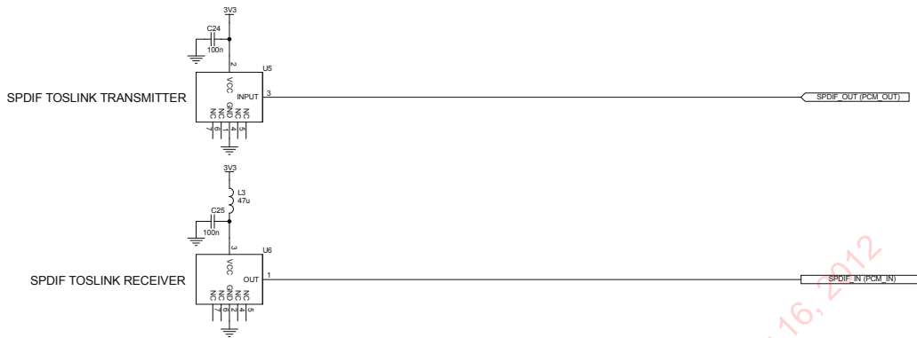
Figure 9.5: Example Circuit for SPDIF Interface (Optical)
