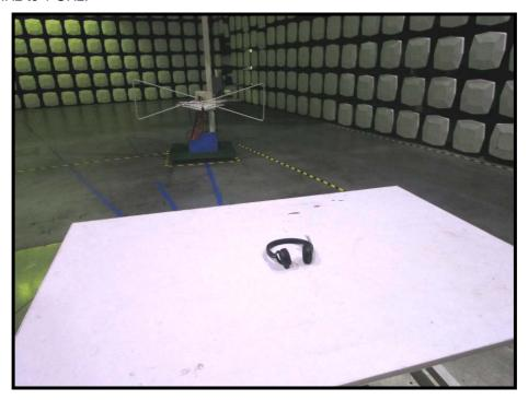
Above 1 GHz: (full anechoic chamber)
