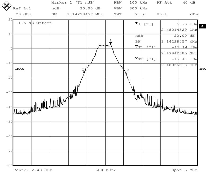
EDR mode (3DH5 data packet with 8DPSK modulation type):
