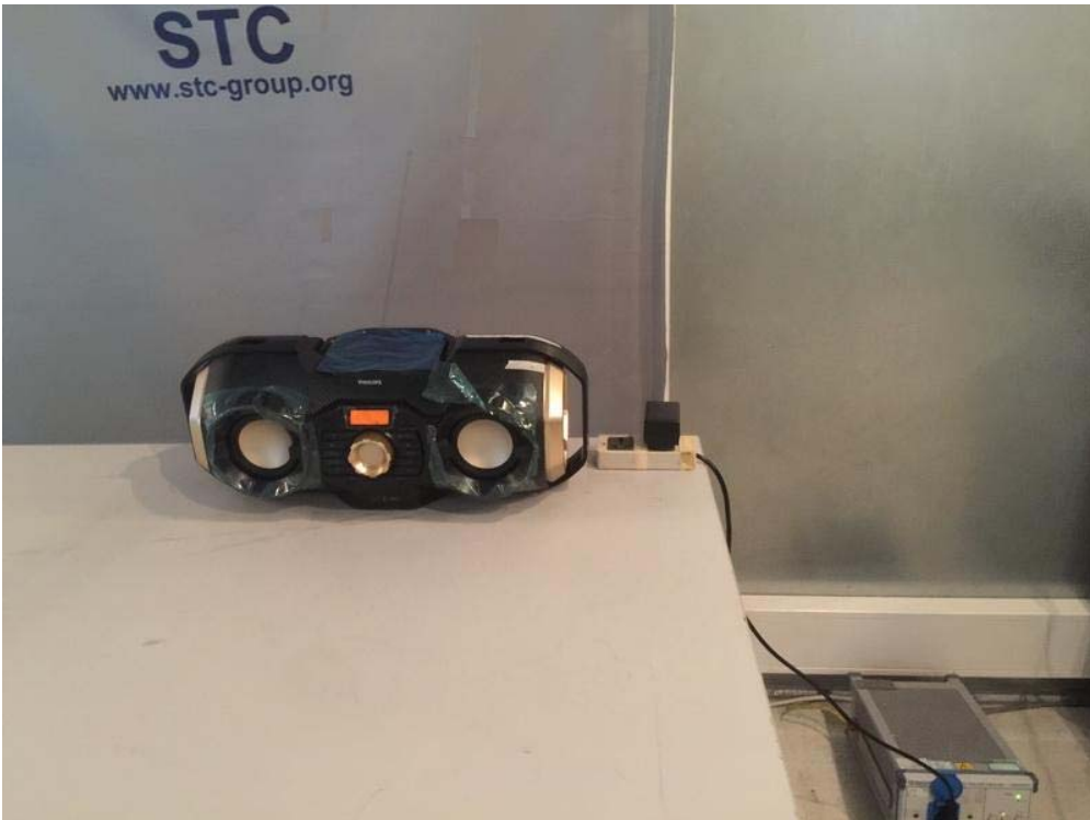
Measurement of Conducted Emission Test Set Up
