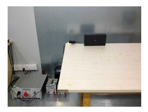
Radiation Emission Test Setup (Below 30MHz)
