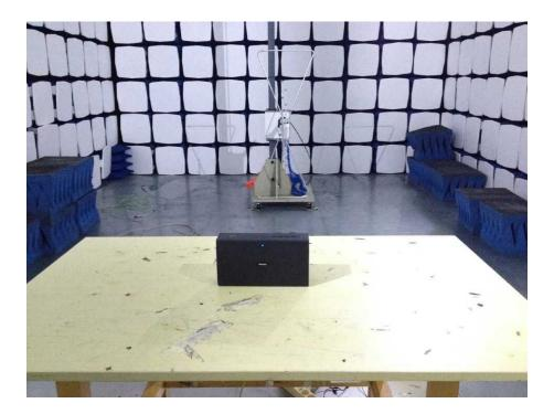
Radiation Emission Test Setup (Above 1GHz)
