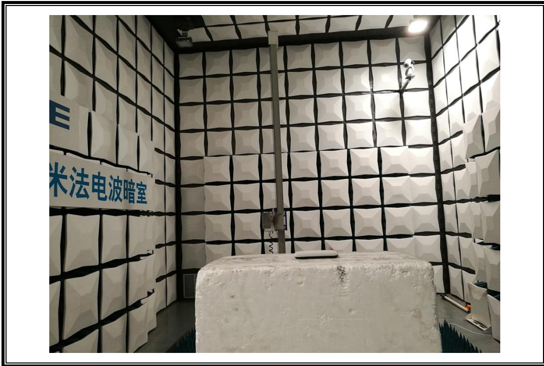
RADIATED RF MEASUREMENT SETUP (ABOVE 1 GHz)
