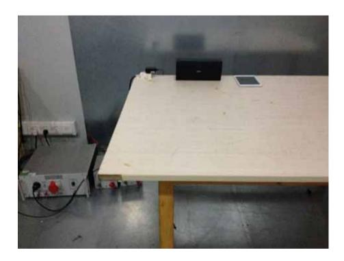
Radiation Emission Test Setup (Below 30MHz)
