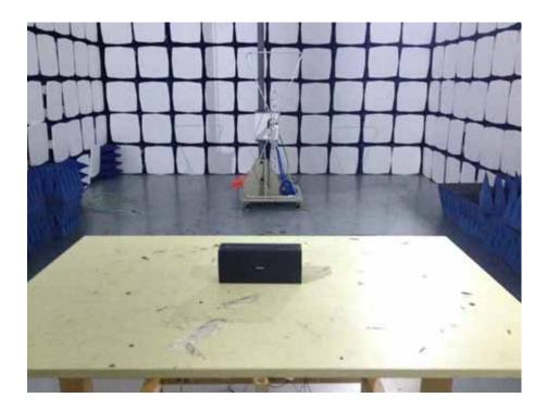
Radiation Emission Test Setup (Above 1GHz)
