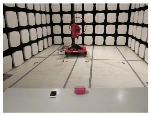
Measurement of Radiated Emission Test Set Up
