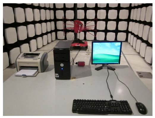
**Measurement of Radiated Emission Test Set Up**
