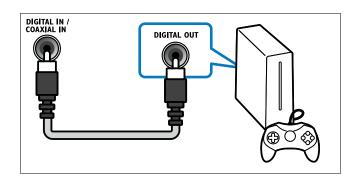
1 Using a coaxial cable, connect the COAXIAL connector on your SoundBar to the COAXIAL/DIGITAL OUT connector on the TV or other device.
