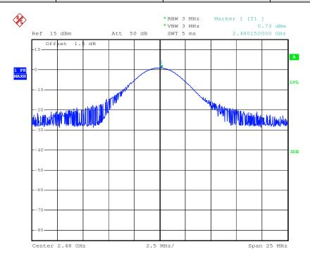
Test mode: π/4DQPSK Test channel: Lowest
