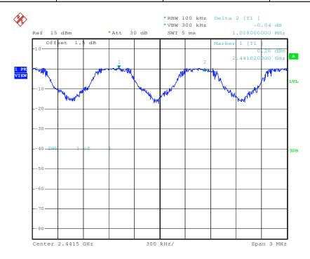
Test mode: π/4DQPSK Test channel: Middle
