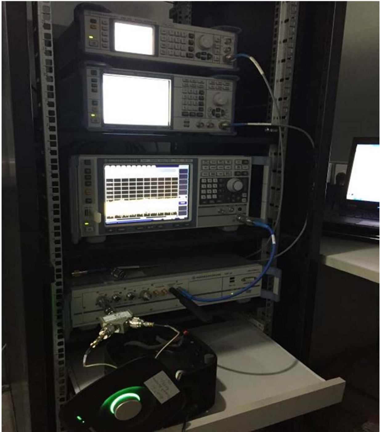
Figure 2 Conducted measurement Test setup for WiFi test
