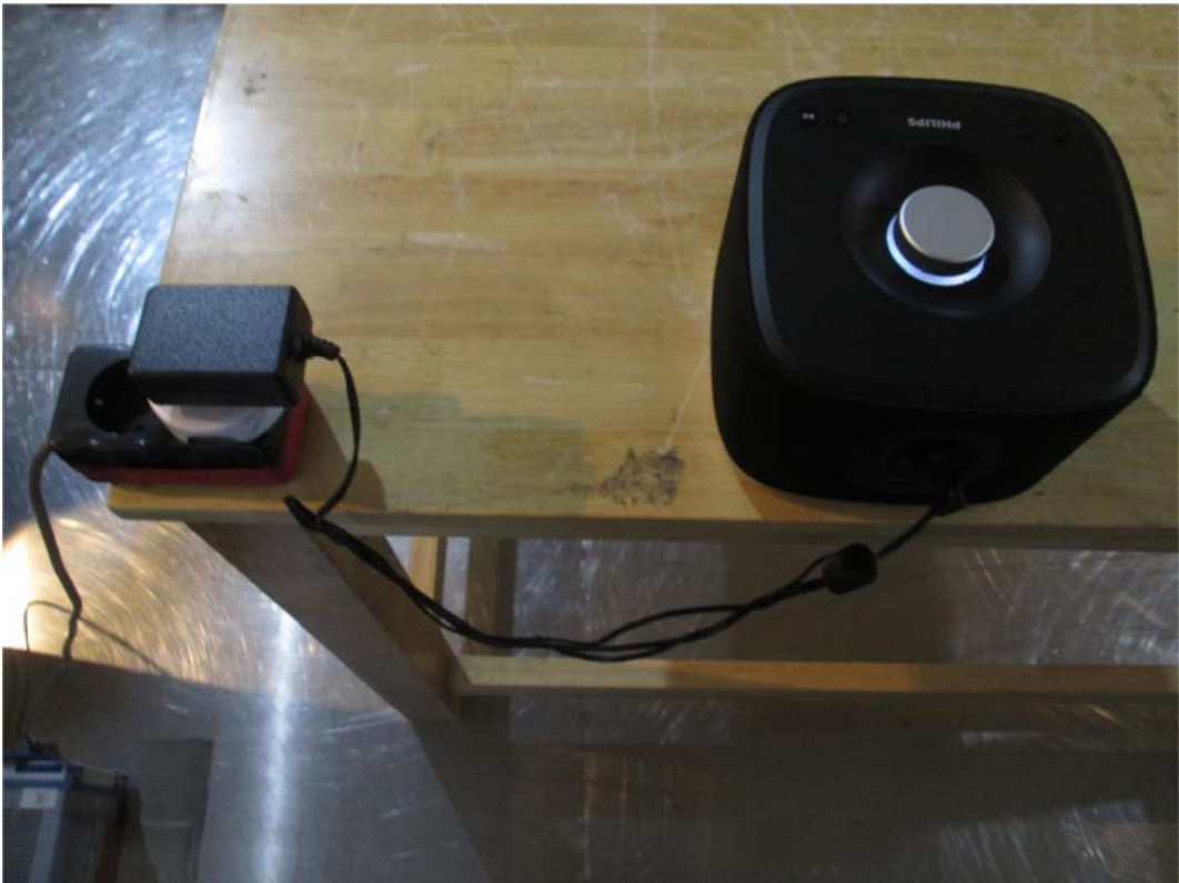
Figure 3 Conducted Emission test setup
