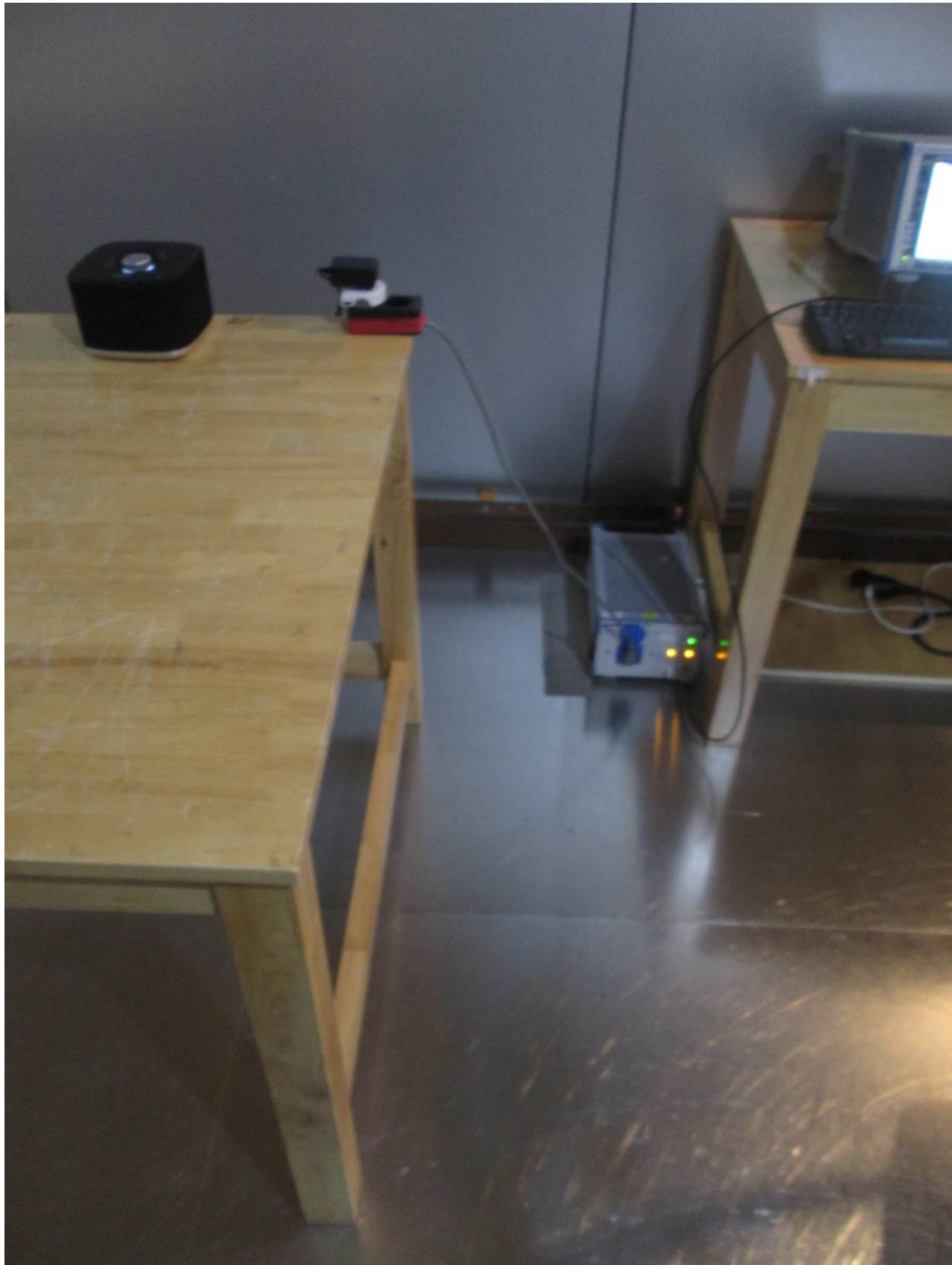
Figure 3 Conducted Emission test setup
