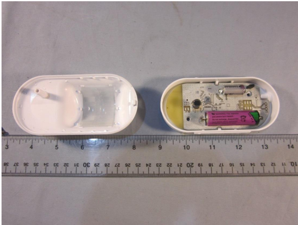
VSW1301 Wall Mount Occupancy/Vacancy Sensor, Top Cover Removed, Internal View
