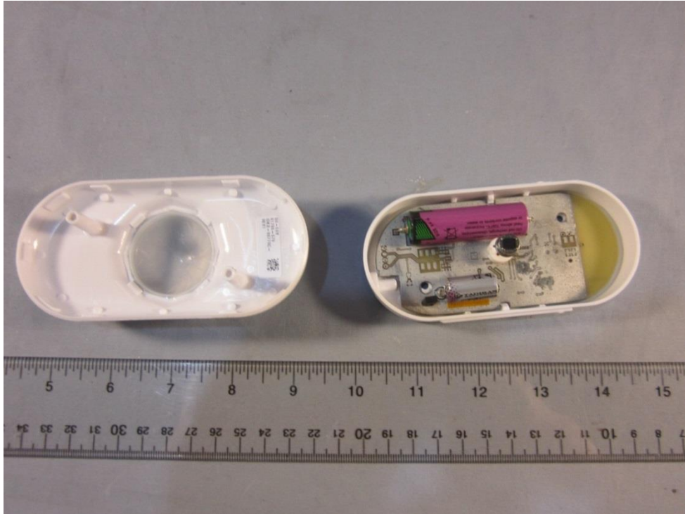
VSC1302, Ceiling Mount Occupancy/Vacancy Sensor, Cover W/Radome Removed
