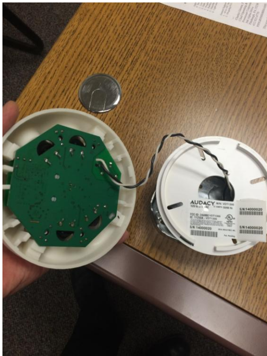
1 - Enclosure opened to access power and to mount backplate (necessary for installation & use)
