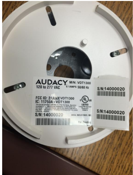
2 - Close-up of backplate and label location. User must separate backplate and expose label to access power and install device.
