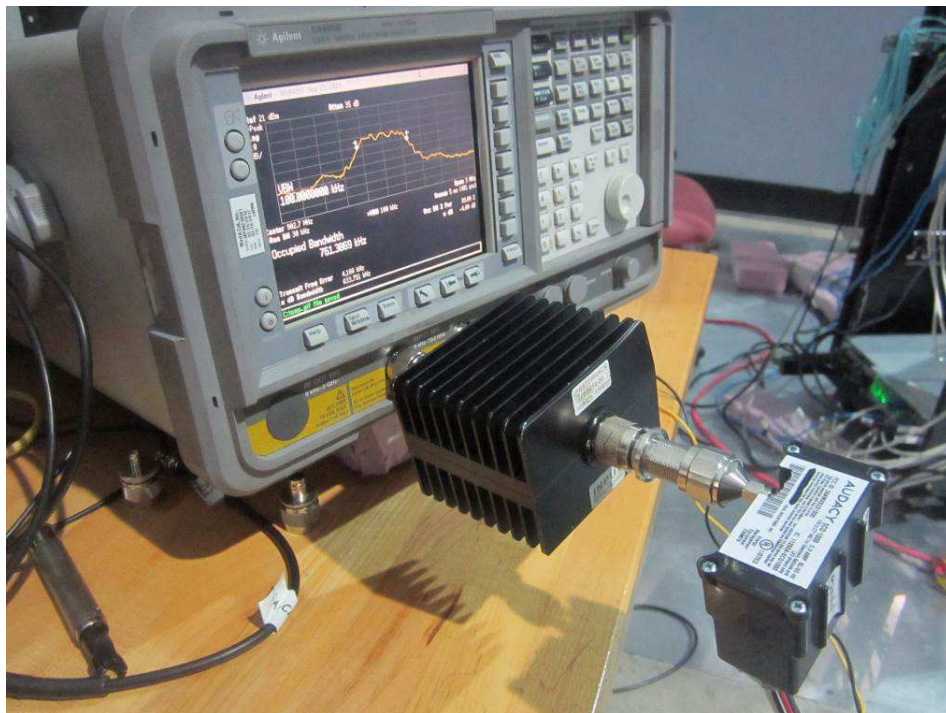
Conducted Testing at Antenna port (Closed up View)
