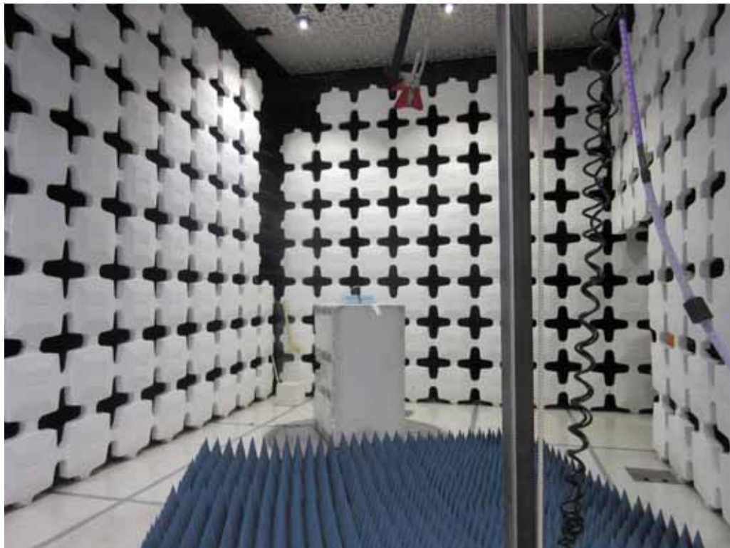
Test Setup for Radiated Emissions (Transmitter) – 1 to 10GHz, Vertical Polarization
