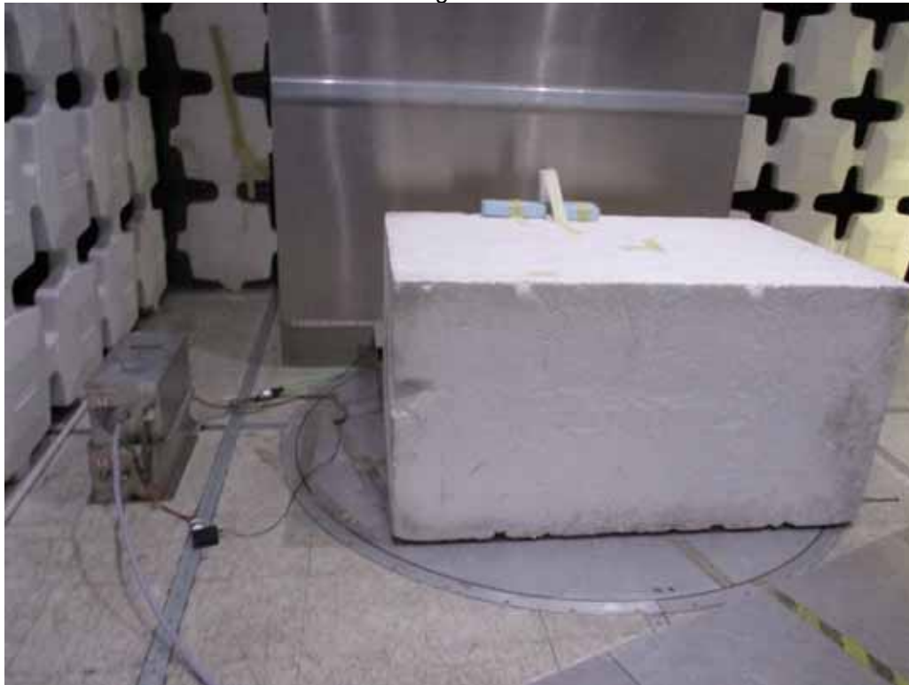
Test Setup for Conducted Emissions
