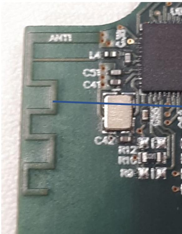
Antenna as integrated on the PCB
