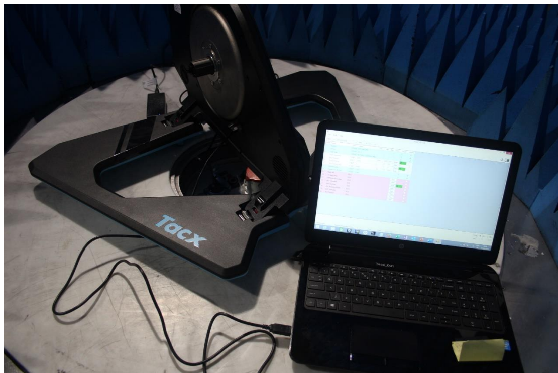
Figure 3: Test Setup Photos – radiated tests and programming
