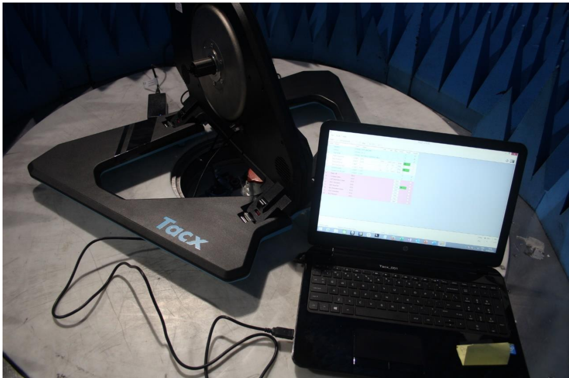
Figure 3: Test Setup Photos – radiated tests and programming
