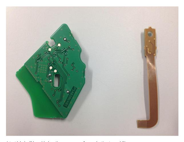
A test label will be added on the copper area for production traceability
