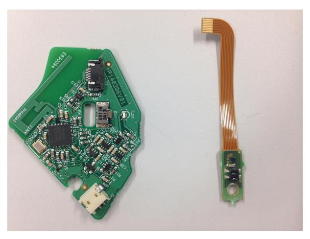
Left is the main board with microcontroller and RF circuit.
