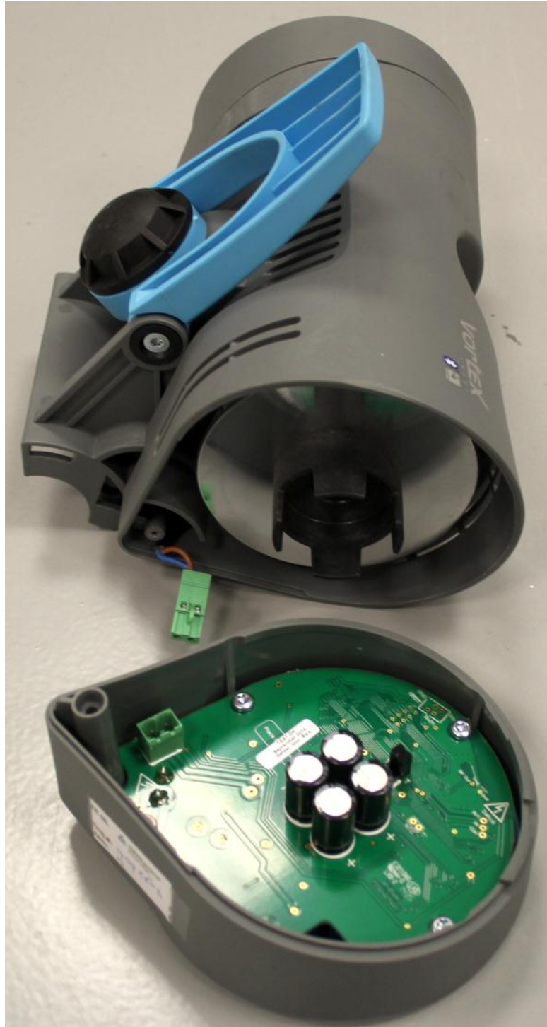
Left side unit, holding the transmitters, removed from main unit
