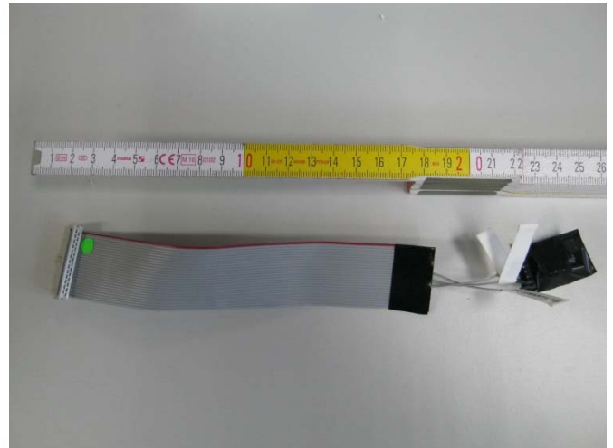
Photograph 2.3-6: Connector cable with USB to serial converter and connector to the RF PCB used for the mode CW and modulated for test purpose, only
