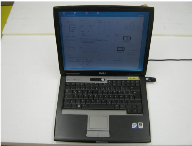
Photograph 2.3-1: Laptop PC with application software and ANT USB Stick used for test mode running
