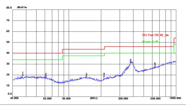
Site #2 3m Anechoic Chamber Polarization: Horizontal Temperature: 25.3(C) Humidity: 56 %
