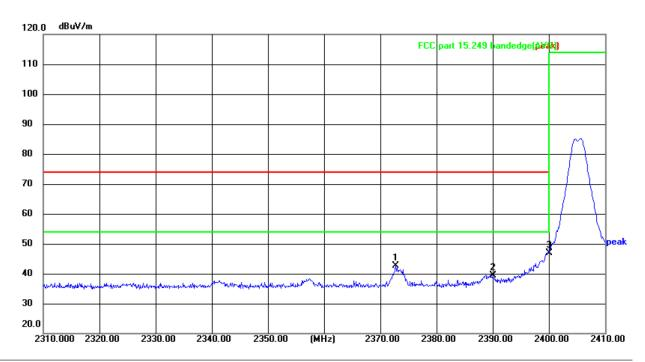
Site Polarization: Vertical Temperature: 24( $^{\circ}$ ) Limit: FCC part 15.249 bandedge(peak) Power: DC 1.5  $^{\lor}$  Humidity: 52  $^{\circ}$
