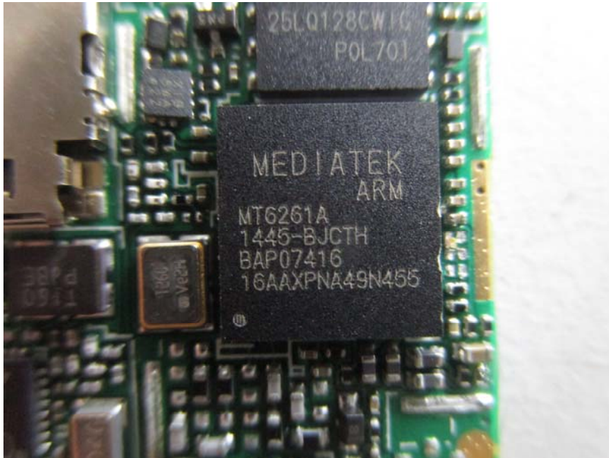
EUT – Main Chip View
