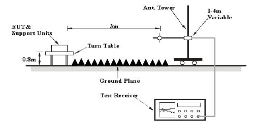
The radiated emission tests were performed at the 3 meters chamber test site, using the setup accordance with the ANSI C63.4-2014. The specification used was the FCC Part 15.109 Class B limits.
