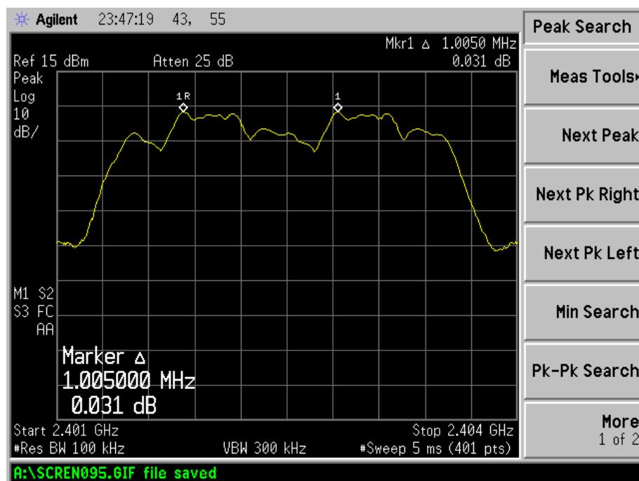
Channel Spacing (Middle CH=1MHz)
