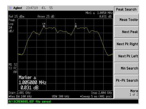
Channel Spacing (Middle CH=1MHz)
