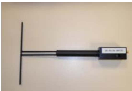
Figure 1 – Satimo COMOSAR Validation Dipole
