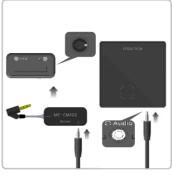
Connect the MOS Kit, BT-Transceiver II wit h the XCAL-Solo III.
