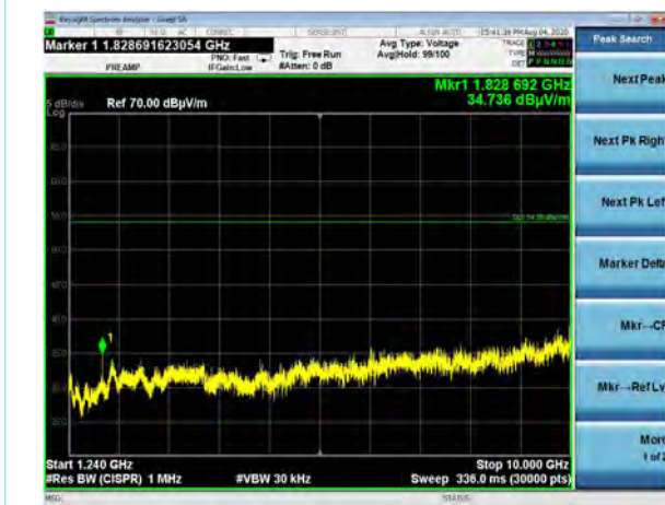
1.24-10 GHz, Horizontal Antenna, Low Ch, 500k, DR4, EUT Vertical
