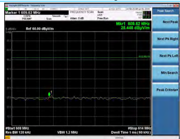
608-614 MHz, Horizontal Antenna, Low Channel DR4, Power Setting 14
