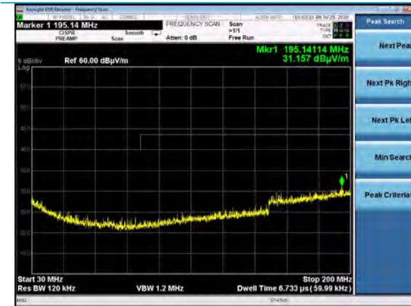
30-200 MHz, EUT Side, Hopping, DR3 Horizontal Antenna, Power Setting 14
