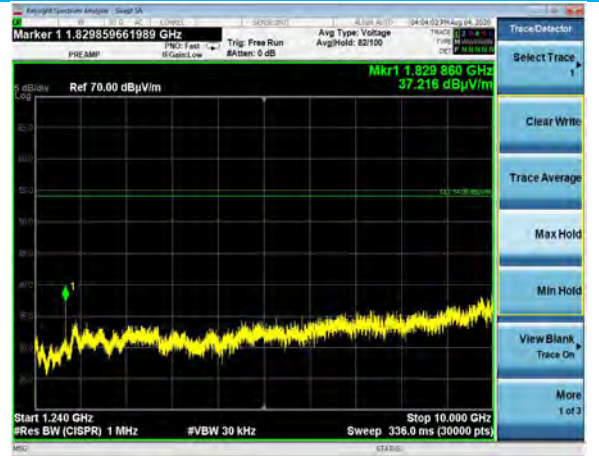
1.24-10 GHz, EUT Vertical, High Channel Horizontal Antenna, DR3, Power Setting 14 Reduced VBW
