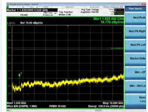
1.24-10 GHz, Vertical Antenna, Low Ch, 500k, DR4, EUT Vertical
