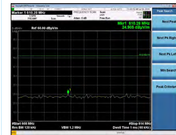
608-614 MHz, Vertical Antenna, High Channel DR4, Power Setting 14
