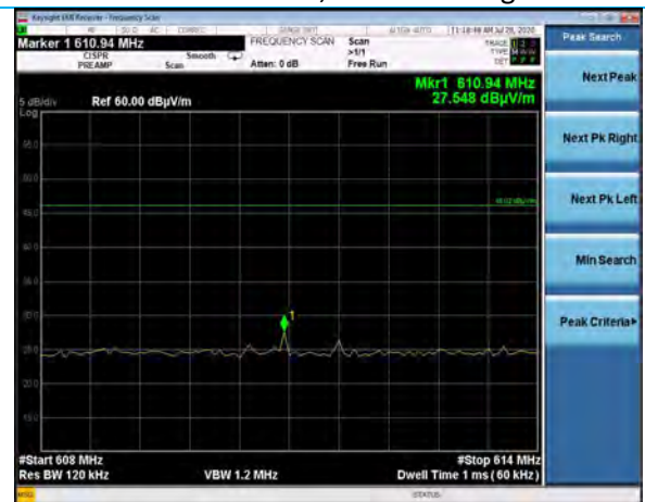
608-614 MHz, EUT Side, Hopping, DR3 Vertical Antenna, Power Setting 14
