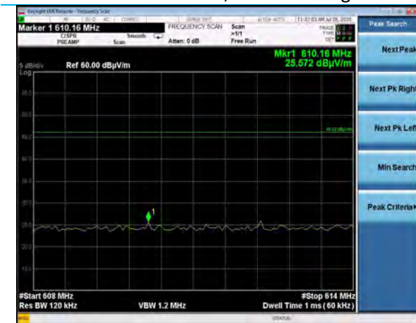
608-614 MHz, EUT Side, Hopping, DR3 Horizontal Antenna, Power Setting -17
