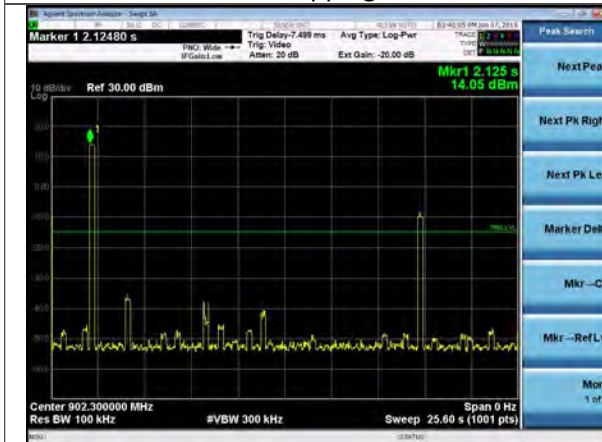
Hops per 25.6s, DR3 Maximum Power Adjacent channel showing up near the end of the sweep. Trigger level was not set high enough.
