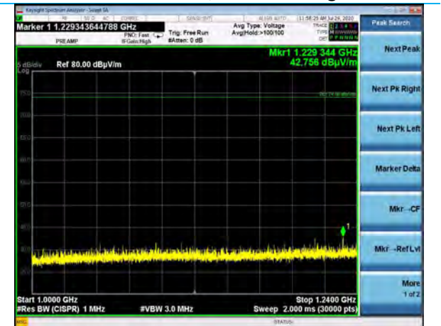
1000-1240 MHz, EUT Side, High Channel, DR3, Vertical Antenna, Power Setting -17
