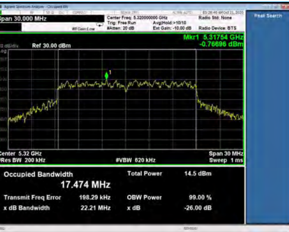
99% Occupied Bandwidth, Channel 64 802.11n, MCS7
