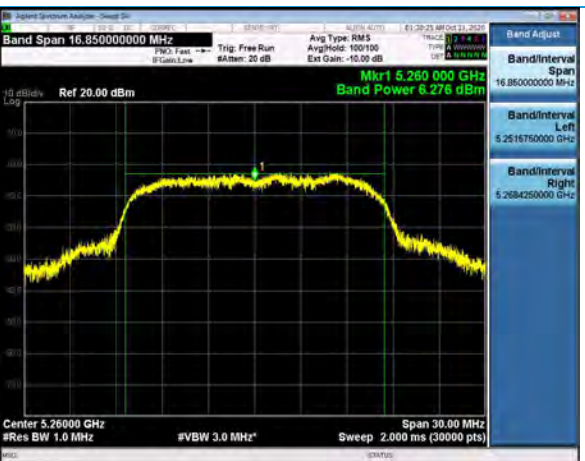
Output Power, Channel 52, 802.11a, 6Mbps
