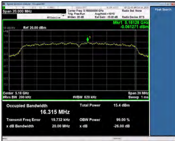
26 dB Emission Bandwidth, Channel 36 802.11a, 6Mbps
