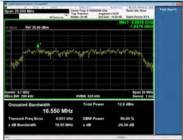
26 dB Emission Bandwidth, Channel 140 802.11a, 54Mbps
