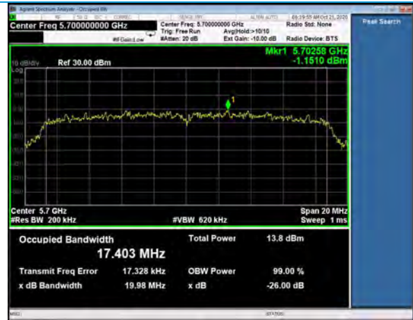
26 dB Emission Bandwidth, Channel 140 802.11n, MCS0
