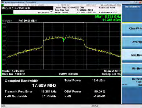
6 dB Emission Bandwidth, Channel 149 802.11n, MCS0
