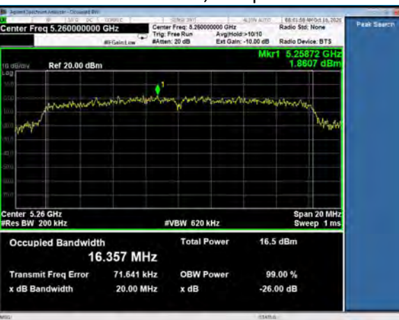
26 dB Emission Bandwidth, Channel 52 802.11a, 6Mbps
