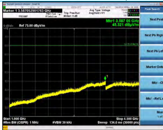
1000-4500 MHz, Horizontal Antenna, Flat EUT Channel 48, 802.11a 6Mbps
