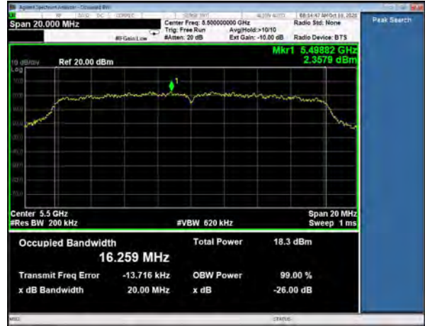
26 dB Emission Bandwidth, Channel 100 802.11a, 6Mbps
