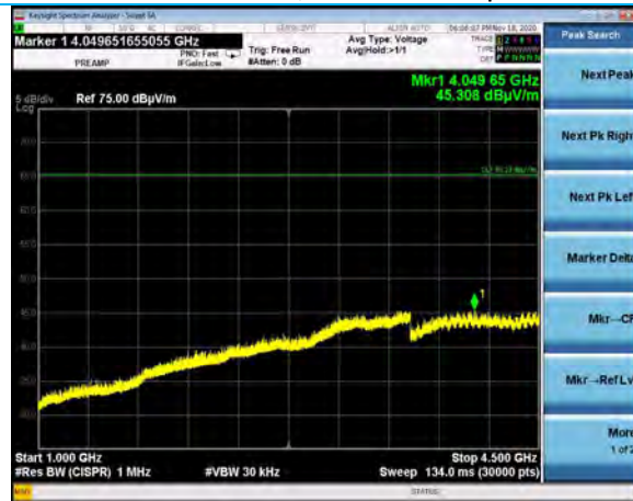
1000-4500 MHz, Vertical Antenna, Flat EUT Channel 48, 802.11a 6Mbps
