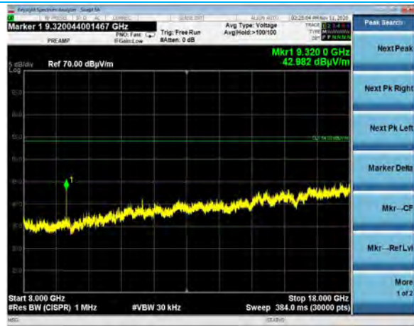
8-18 GHz, Vertical Antenna, Flat EUT Channel 165, 6Mbps
