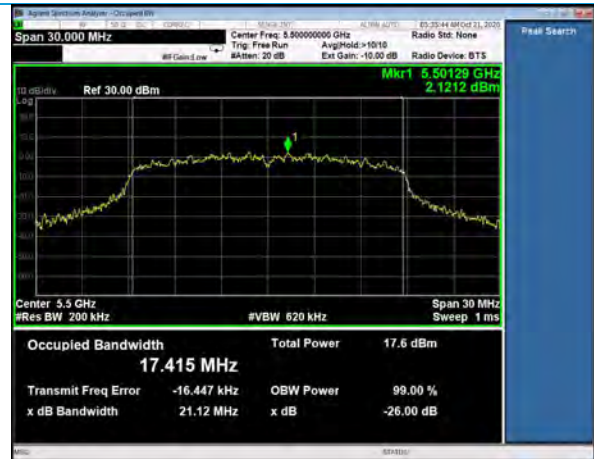
99% Occupied Bandwidth, Channel 100 802.11n, MCS0
