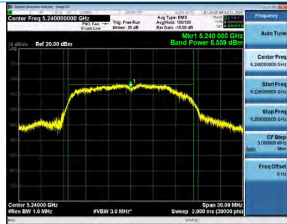
Output Power, Channel 48, 802.11a, 6Mbps
