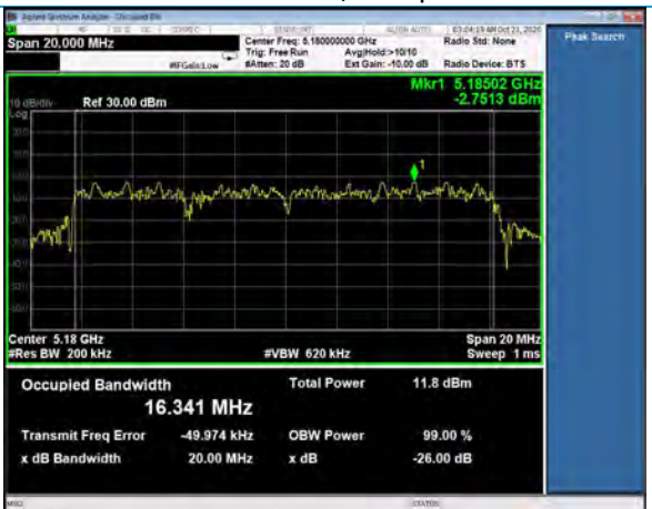
99% Occupied Bandwidth, Channel 36 802.11a, 6Mbps
