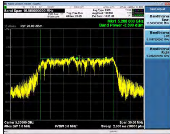
Output Power, Channel 40, 802.11a, 54Mbps
