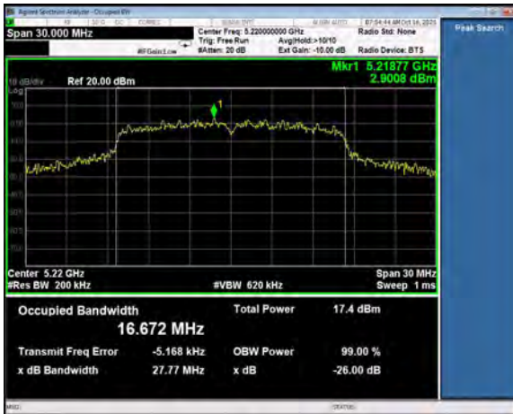
99% Occupied Bandwidth, Channel 44 802.11a, 6Mbps
