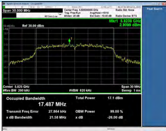
99% Occupied Bandwidth, Channel 165 802.11n, MCS0
