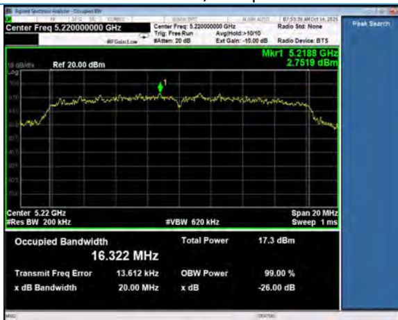
26 dB Emission Bandwidth, Channel 44 802.11a, 6Mbps
