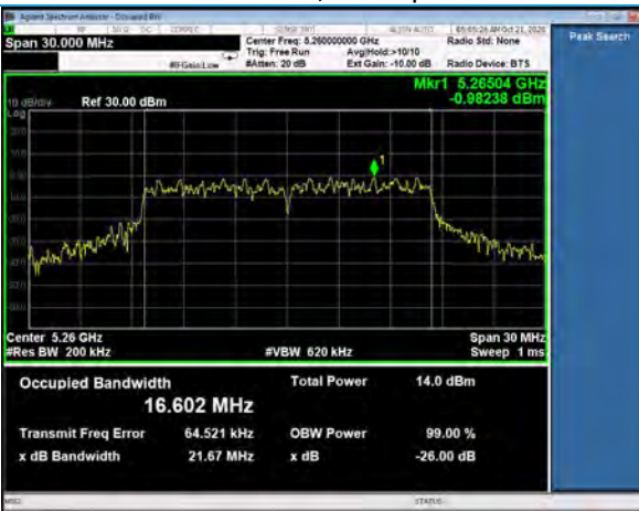
99% Occupied Bandwidth, Channel 52 802.11a, 54Mbps
