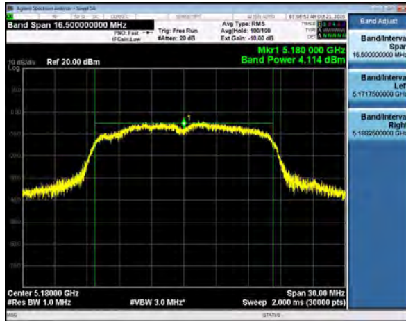
Output Power, Channel 36, 802.11a, 6Mbps
