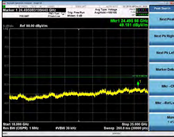
18-25 GHz, Horizontal Antenna, Vertical EUT Channel 165, 6Mbps
