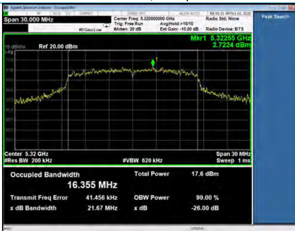
99% Occupied Bandwidth, Channel 64 802.11a, 6Mbps
