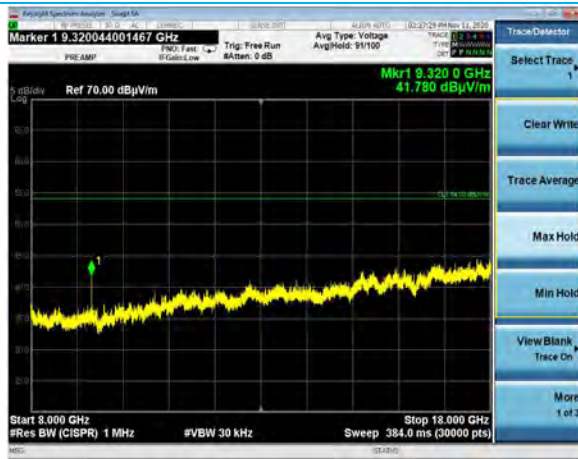
8-18 GHz, Horizontal Antenna, Flat EUT Channel 165, 6Mbps
