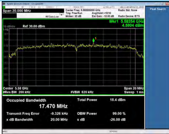
26 dB Emission Bandwidth, Channel 116 802.11n, MCS0
