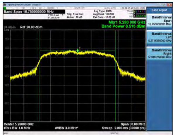
Output Power, Channel 56, 802.11a, 6Mbps
