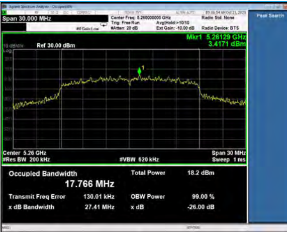
99% Occupied Bandwidth, Channel 52 802.11n, MCS0
