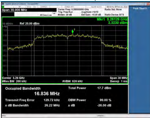
99% Occupied Bandwidth, Channel 52 802.11a, 6Mbps
