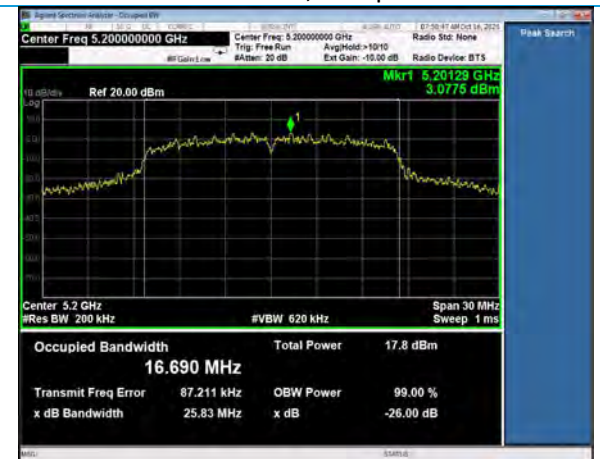
99% Occupied Bandwidth, Channel 40 802.11a, 6Mbps
