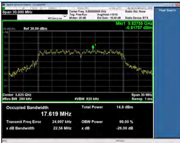
99% Occupied Bandwidth, Channel 165 802.11n, MCS7
