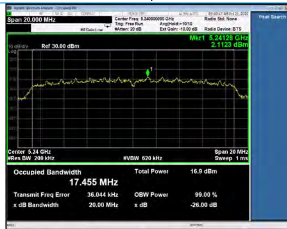
26 dB Emission Bandwidth, Channel 48 802.11n, MCS0
