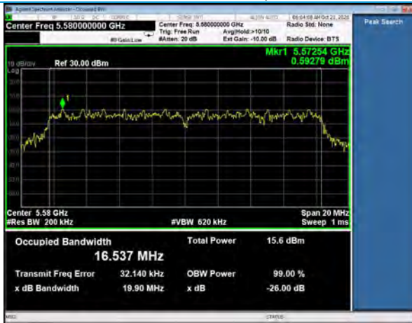
26 dB Emission Bandwidth, Channel 116 802.11a, 54Mbps
