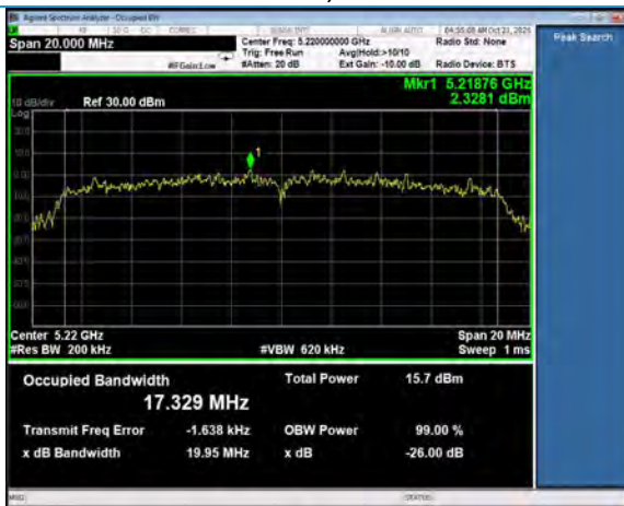
26 dB Emission Bandwidth, Channel 44 802.11n, MCS0
