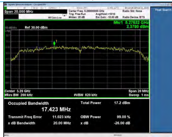
26 dB Emission Bandwidth, Channel 56 802.11n, MCS0
