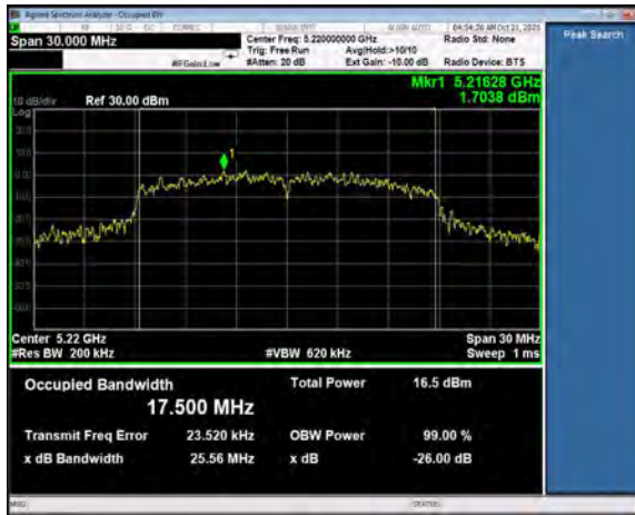
99% Occupied Bandwidth, Channel 44 802.11n, MCS0
