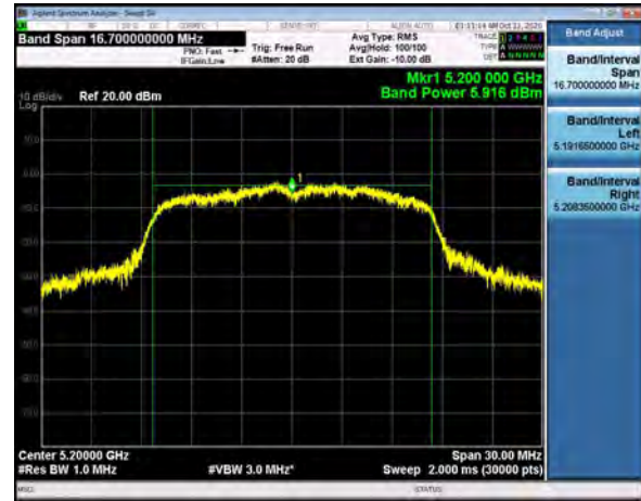
Output Power, Channel 40, 802.11a, 6Mbps
