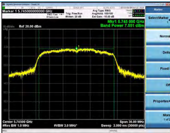
Output Power, Channel 149, 802.11a, 6Mbps
