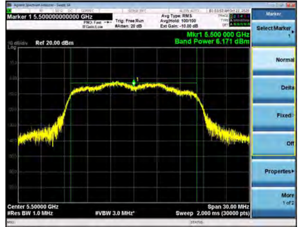
Output Power, Channel 100, 802.11a, 6Mbps
