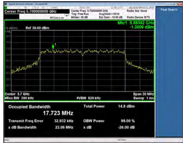
99% Occupied Bandwidth, Channel 140 802.11n, MCS7
