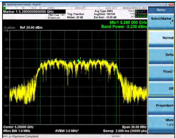
Output Power, Channel 56, 802.11a, 54Mbps
