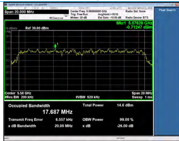
26 dB Emission Bandwidth, Channel 116 802.11n, MCS7
