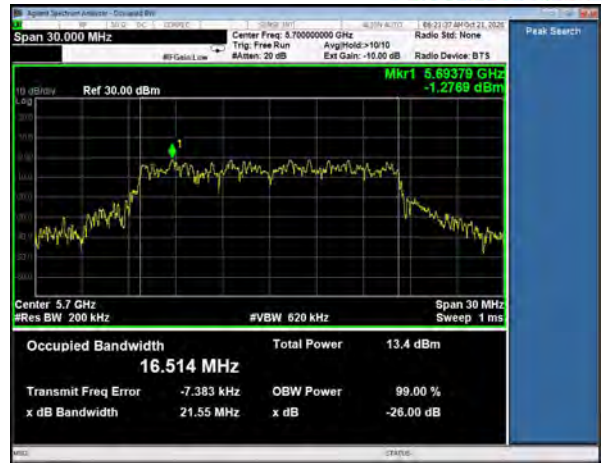
99% Occupied Bandwidth, Channel 140 802.11a, 54Mbps
