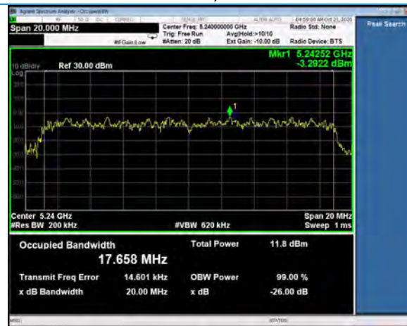
26 dB Emission Bandwidth, Channel 48 802.11n, MCS7
