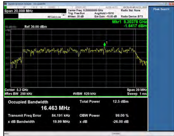
26 dB Emission Bandwidth, Channel 40 802.11a, 54Mbps
