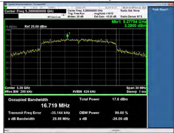
99% Occupied Bandwidth, Channel 56 802.11a, 6Mbps
