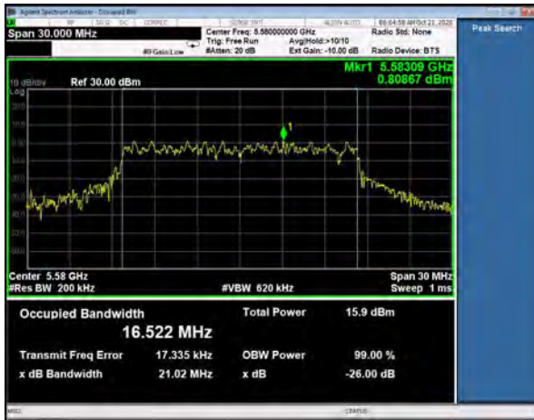
99% Occupied Bandwidth, Channel 116 802.11a, 54Mbps
