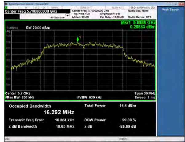
99% Occupied Bandwidth, Channel 140 802.11a, 6Mbps
