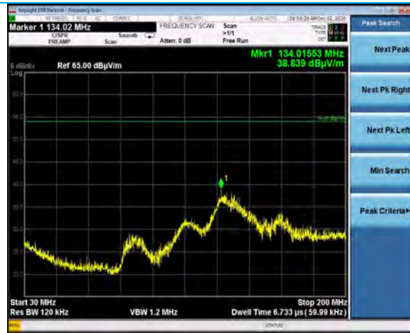
30-200 MHz, Horizontal Antenna, Vertical EUT Channel 36, 802.11a 6Mbps
