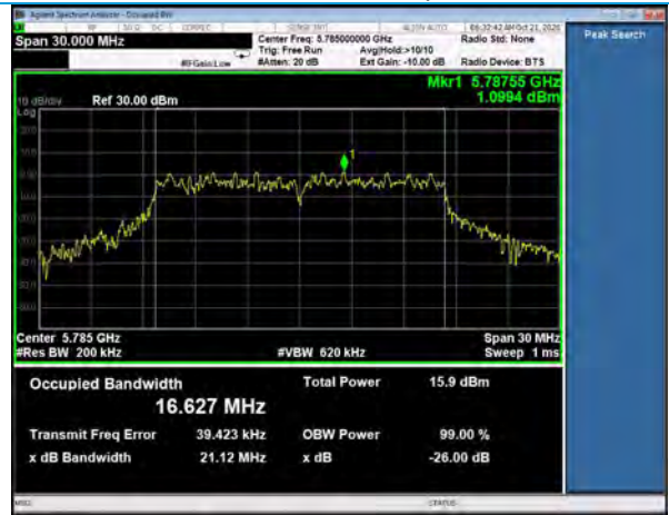
99% Occupied Bandwidth, Channel 157 802.11a, 54Mbps
