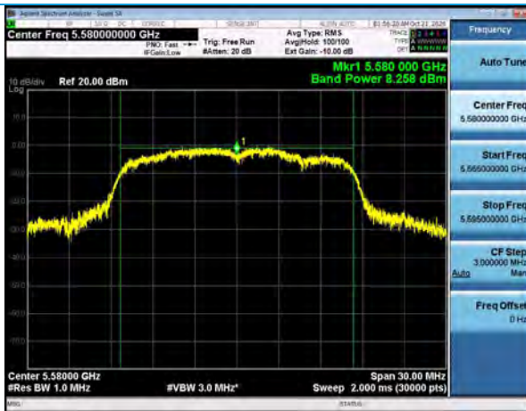
Output Power, Channel 116, 802.11a, 6Mbps
