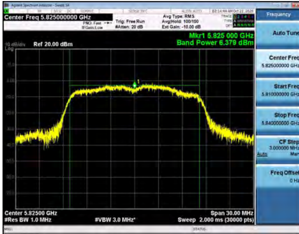
Output Power, Channel 165, 802.11a, 6Mbps
