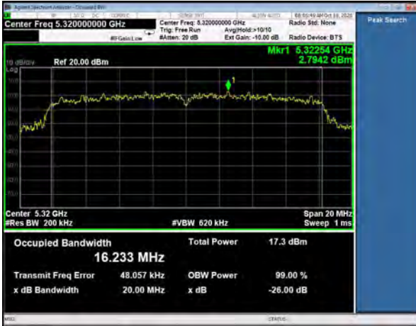
26 dB Emission Bandwidth, Channel 64 802.11a, 6Mbps
