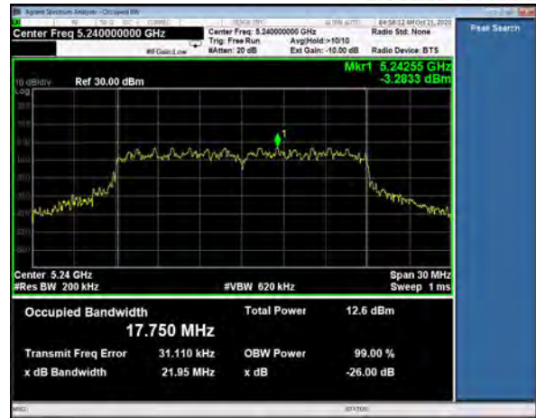
99% Occupied Bandwidth, Channel 48 802.11n, MCS7
