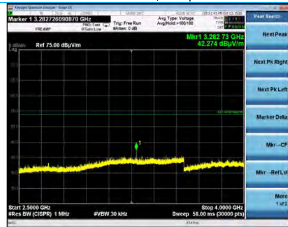
2500-4000 MHz, Vertical Antenna, Vertical EUT Channel 11
