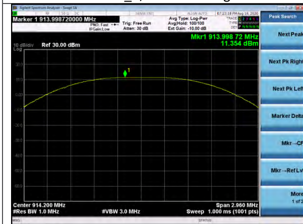
Pout, DR13 High Channel Laird Rev_B, Power Setting 12
