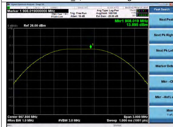
Pout, DR13 Mid Channel Laird Rev_B, Power Setting 18
