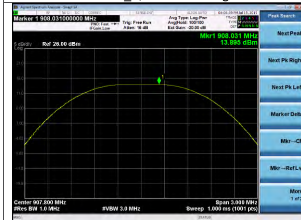
Pout, DR4 Mid Channel Laird Rev_B, Power Setting 18
