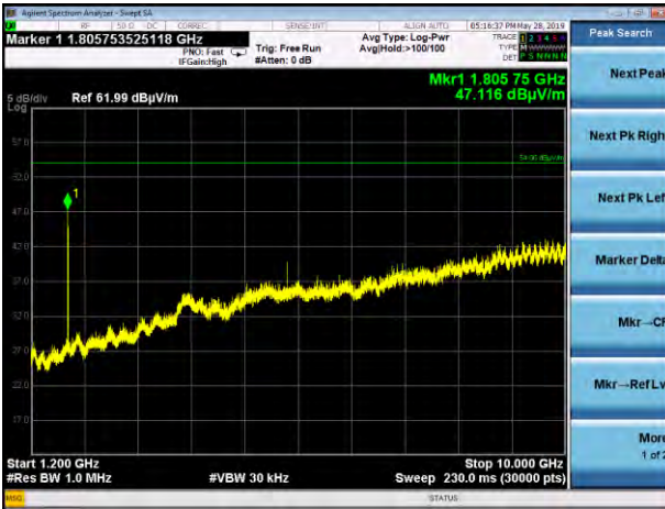
1.2-10 GHz, Horizontal Antenna, Low Ch, 500k, DR4, EUT Flat
