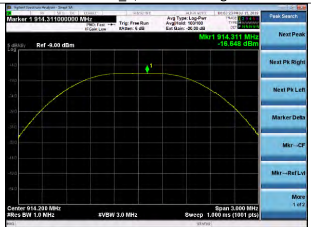
Pout, DR13 High Channel Laird Rev_B, Power Setting -17
