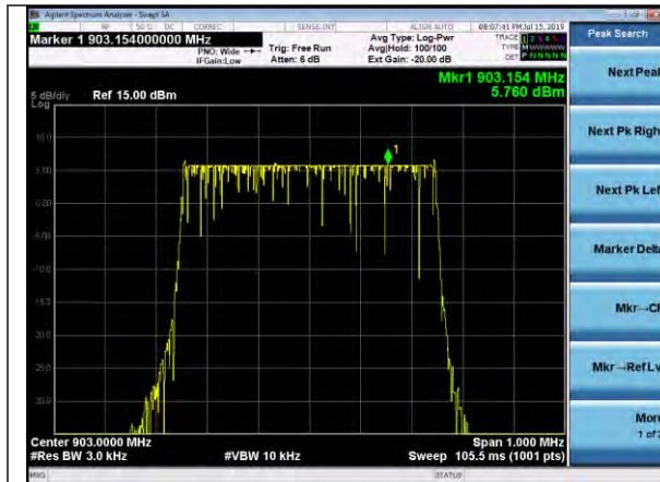
PSD, DR4 Low Channel Laird Rev_B, Power Setting 18
