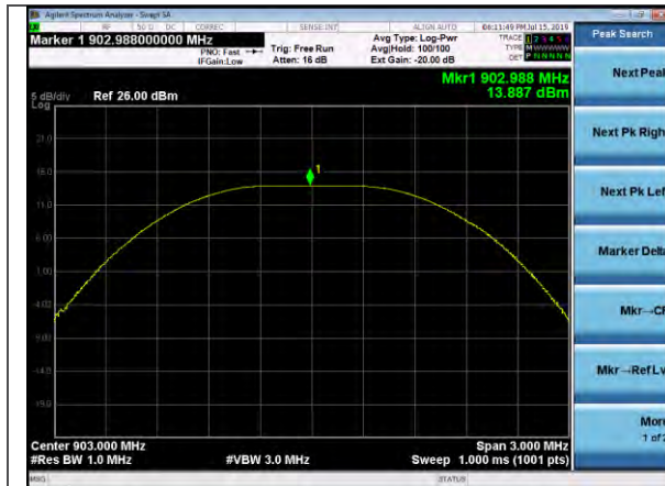
Pout, DR4 Low Channel Laird Rev_B, Power Setting 18
