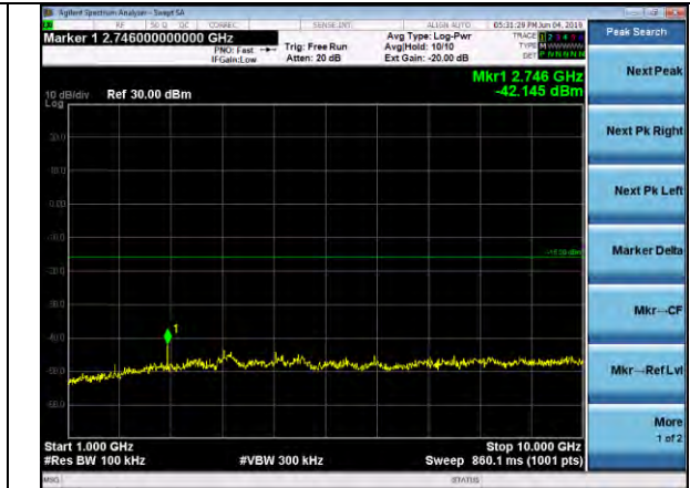
1-10 GHz, DR13 High Channel Laird Rev_B, Power Setting 18
