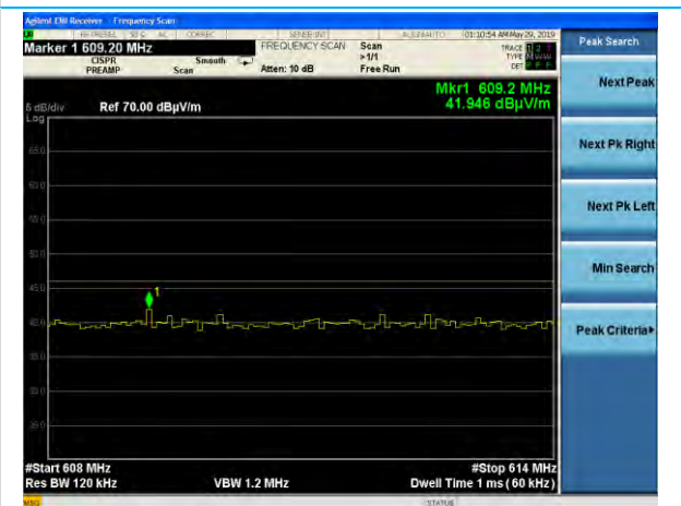
608-614 MHz, Horizontal Antenna, Low Channel, 500kHz, DR13
