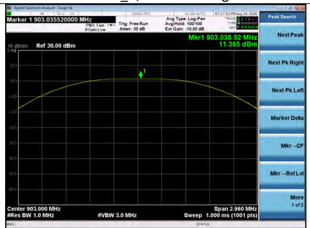
Pout, DR4 Low Channel Laird Rev_B, Power Setting 12
