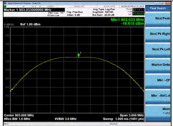
Pout, DR13 Low Channel Laird Rev_B, Power Setting -17
