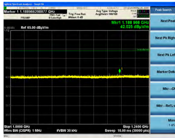
1000-1240 MHz, Horizontal Antenna, High Channel, 500 kHz, DR 13, Reduced VBW
