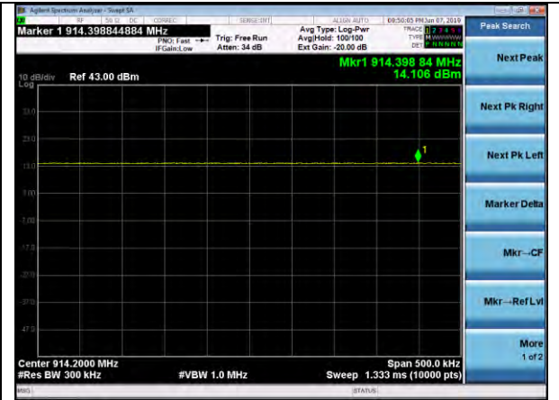
Nominal Power, Low Temp, High Channel
