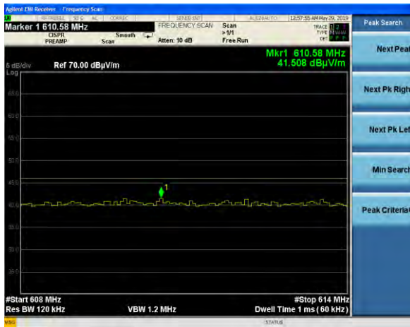
608-614 MHz, Horizontal Antenna, Low Channel, 500kHz, DR4
