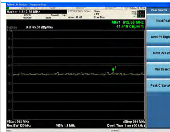
608-614 MHz, EUT Side, Hopping, DR3, Horizontal Antenna, Laird Rev_B, Power Setting 18
