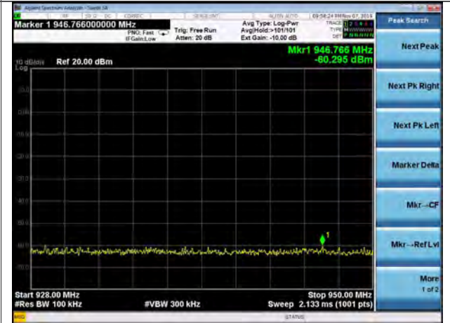
928-950 MHz, Hopping Laird Rev_B, Power Setting 18
