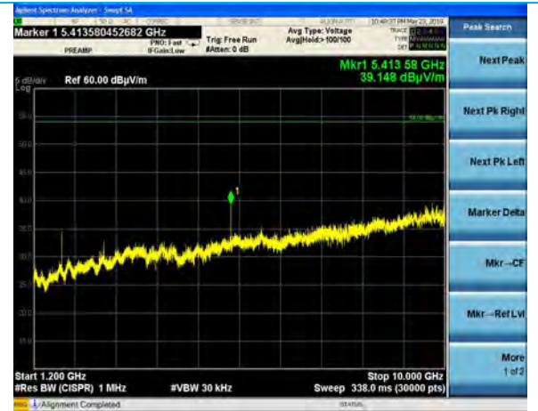
1.2-10 GHz, EUT Vert, Mid Chan, DR0, Horizontal Antenna, Laird Rev_B, Power Setting 18
