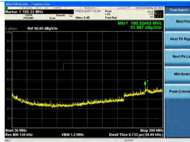
30-200 MHz, EUT Side, Low Chan, DR3, Horizontal Antenna, Laird Rev_B, Power Setting 18
