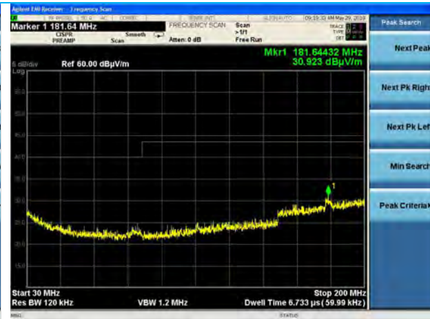
30-200 MHz, EUT Side, Low Chan, DR3, Vertical Antenna, Laird Rev_B, Power Setting 18
