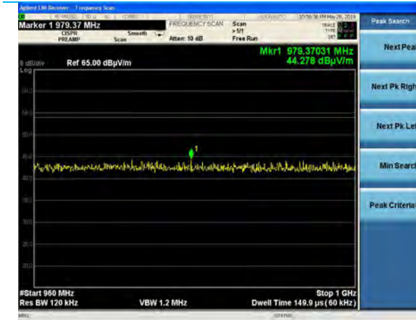
960-1000 MHz, EUT Side, High Chan, DRO, Horizontal Antenna Laird Rev_B, Power Setting 18
