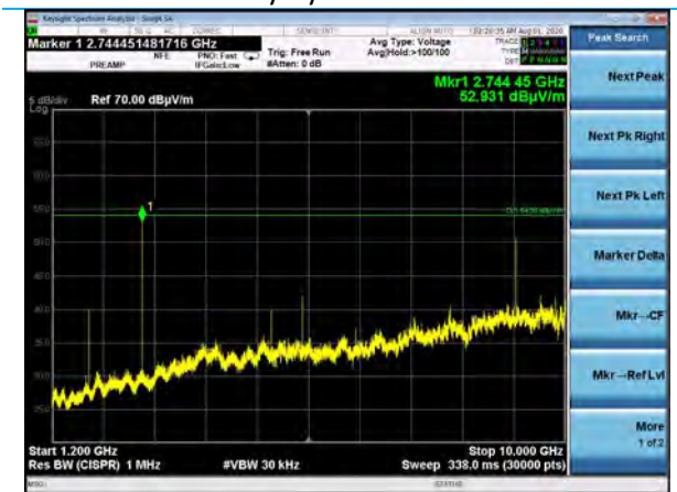
1.2-10 GHz, EUT Vert, Mid Chan, DR3, Vertical Antenna, Laird Rev_B1, Power Setting 12
