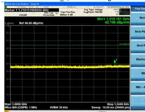
1000-1240 MHz, EUT Side, Hopping, DR3, Horizontal Antenna, Average Antenna, Laird Rev_B, Power Setting 18
