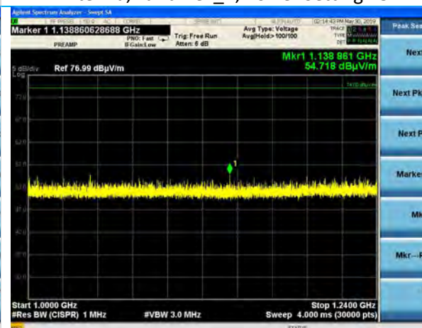
1000-1240 MHz, EUT Side, High Chan, DR3, Horizontal Antenna, Peak Laird Rev_B, Power Setting 18
