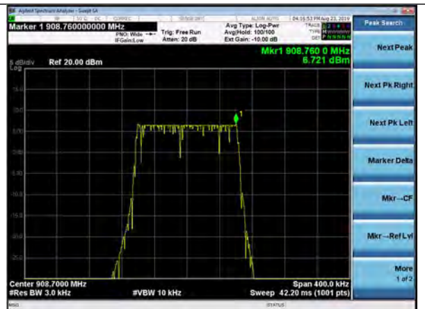
PSD, DR3, 908.7 MHz Laird Rev_B, Power Setting 18
