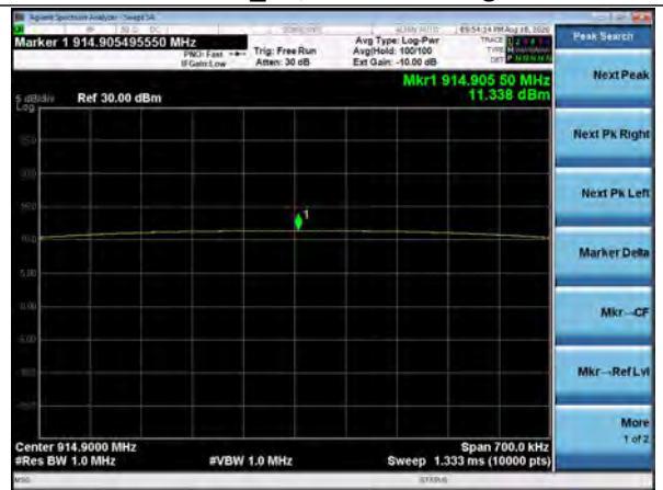
Output Power, DR0, 914.9 MHz Laird Rev_B1, Power Setting 12
