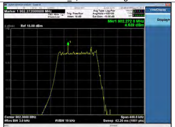
PSD, DR0, 902.3 MHz Laird Rev_B, Power Setting 18
