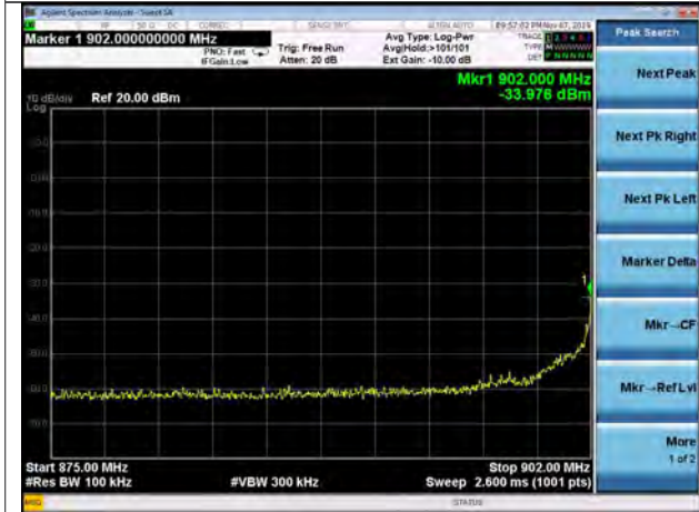
875-902 MHz, Hopping Laird Rev_B, Power Setting 18
